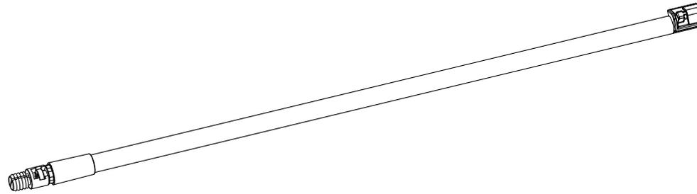
Step 1. Pull to release the sleeve, remove the dowel and screw.
