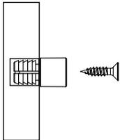
Step 2. Insert expanding dowel into pre-drilled hole on the drawer front.
