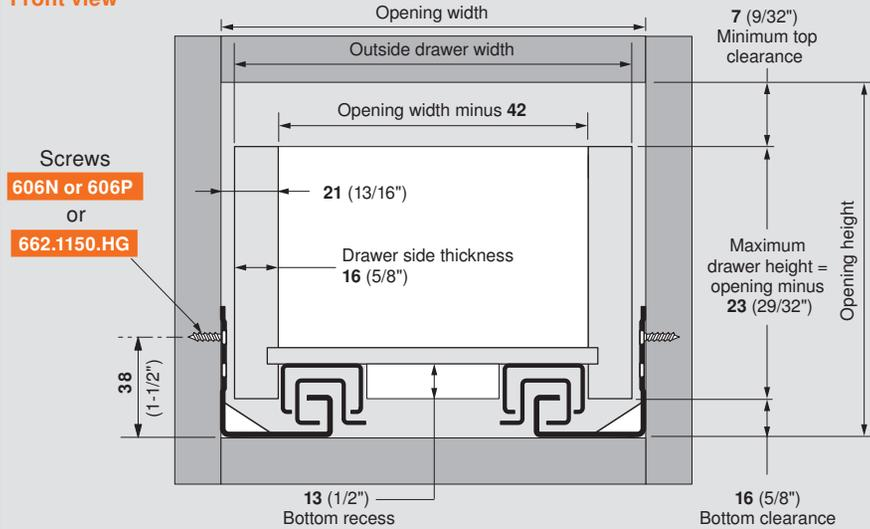
**NOTE:** Drawer side material thickness may vary. Accurate measurement of drawer side material thickness should be used when calculating outside drawer width using the table below. Inside drawer width **must** equal opening width minus 42 (1-21/32") for MOVENTO to align and function optimally.
