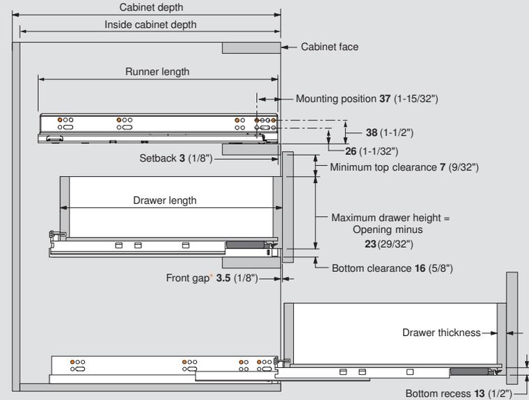
**NOTE\*:** Front gap is 0 without TIP-ON BLUMOTION installed
