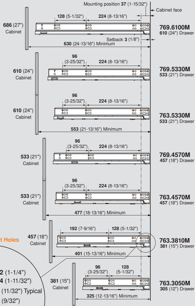
**NOTE:** Orange dots indicate screw locations required to meet specified load capacities
