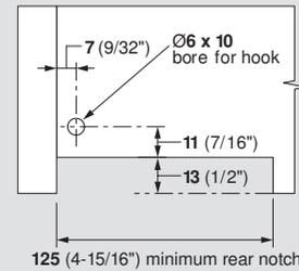
**NOTE:** Use of the T65.1600.01 MOVENTO template is essential for accurate location and angle of pre-bored locking device holes and accurate boring for rear hook holes
