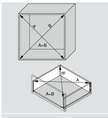
To ensure optimal function with a minimum front gap of **3.5** mm, precise manufacturing is required. Please adhere to our specifications and verify that cabinets and drawers are square.
