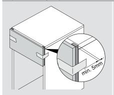
a) clamp a spacer between front and cabinet or
