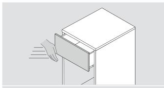
To tension TIP-ON springs, always close drawers with TIP-ON BLUMOTION using adequate force. Reduce the amount of force used accordingly for loaded drawers.
