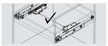
To achieve the optimal trigger range for TIP-ON BLUMOTION, use a synchronization rod with synchronization adapters.
