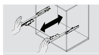
In order to prevent damage to the synchronization adapters, open or close concealed runners in parallel with one another once the synchronization components have been installed.
