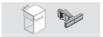
The front gap should be adjusted identically on each side to a minimum of **3.5** mm.
