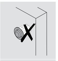
Do not use bumpers, as this can inhibit the function of TIP-ON BLUMOTION when the drawer front is pressed.
