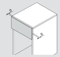
b) adjust the front gap to 0 mm or
