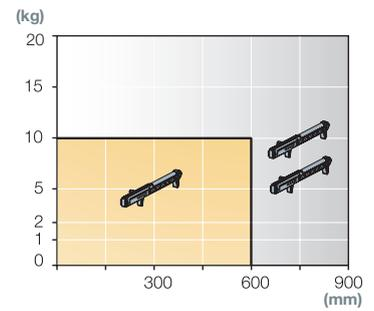
Mount 1 or 2 mechanisms depending on drawer weight and width
