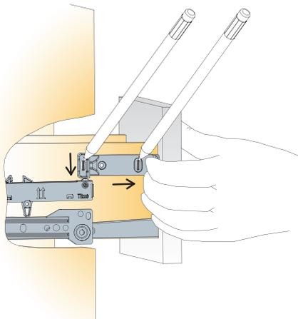
Align the activator with the top of the mechanism and fix with two screws
