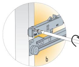
Screw the mechanism to the face frame
