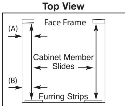
**Step 5:** Mount Rear Bracket. Extend the slide rear mounting bracket until it contacts the rear (Furring Strip). Bottom of slide should be  $13\frac{3}{8}$ " from cabinet floor. Rear mounting bracket should be the same distance from the side cabinet wall at rear of slide as it is up front. Drive mounting screw in center horizontal slot of rear mounting bracket, tighten. Tighten screw in front bracket.
