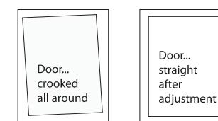
**Step 9:** If your cabinet door is not straight (even all around) you can adjust it by loosening the screws on one of the sides, properly align the cabinet door and re-tighten the screws.
