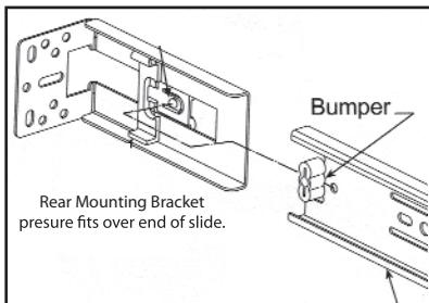
**Step 1:** Install rear bracket to rear of slide.
