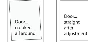
**Step 8:** Pull door open from sides of door at slide level. (See illustration 7). Make sure to securely tighten top screws.
